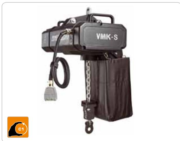
The VMK-S hoists according to BGV C1, DIN 56950:2012-05 and EN 61508 SIL 3 are notable for their innovative feature set and unusually flexible handling, whilst satisfying at all times the highest standards of safety. Particularly remarkable are the two independent, low-noise and maintenance-free brakes with air gap monitoring, a real-time load-measuring
