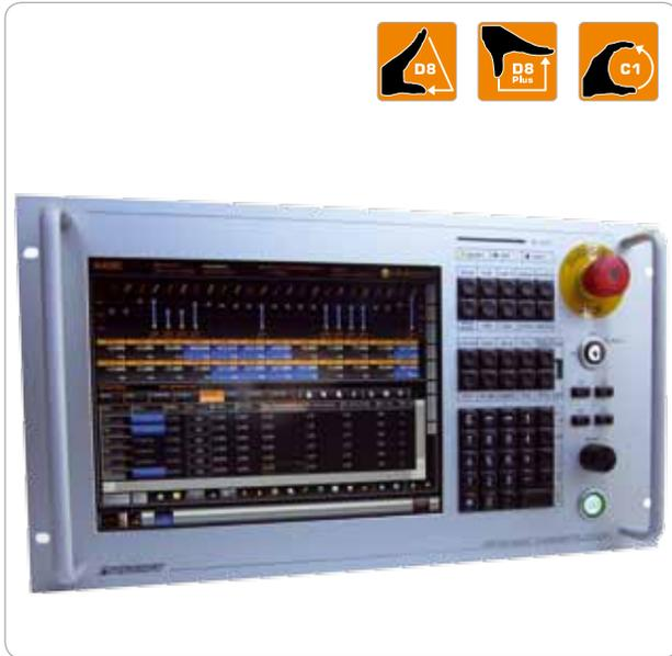
The I-Motion Basic-S Show Controller is based on the tried-and-tested Basic controller and constitutes a compact System Controller for the systemic control of kinetic drives in mobile and flexible project applications with extended ancillary features. The additional features are the general dual-channel implementation according to EN 61508 SIL 3, the User ID chip card function as well
